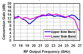
Vd = 5V, Idq = 425mA, Vmxr = Vdbl = -0.9V IF = 2GHz +/- 5MHz @ -8dBm Input/Tone, +2dBm LO
